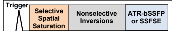
Figure 1. MIR pulse sequence. Selective spatial saturation resets magnetization. Nonselective inversions suppress a range of background T 1 species. ATR-bSSFP or SSFSE readout maintains contrast.
