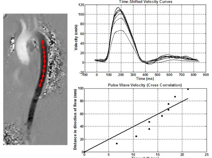
Fig 3. XC method. Flow patterns (up) are computed at several points along the aortic path (left). Cross correlation is used to estimate time shifts between consecutive points, from which PWV is computed by line fitting (down).
