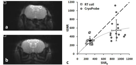
**Figure 1:** Representative GE-EPI images acquired using RT coil (a) and CryoProbe (b), respectively. Dashed circles indicate left and right somatosensory areas (S1), while squares were selected for raw image noise estimation. (c) Temporal SNR (tSNR) plotted versus image SNR (SNR<sub>0</sub>). Dashed line represents line of equity, while gray line indicates the result of linear least-squares fitting according to [4] ( $\lambda=0.00144$ ,  $R^2=0.94$ ).
