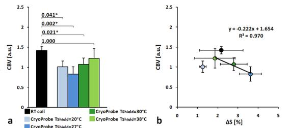
**Figure 3:** (a) CBV measurements using the RT coil (N=4) and the CryoProbe at T<sub>Shield</sub>=20°C (N=3), 27°C (N=3), 30°C (N=10), and 38°C (N=3). (b) Correlation between CBV and maximum BOLD signal response. Solid line represents linear regression of the CryoProbe values for T<sub>Shield</sub>=27 - 38°C.
