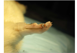
Fig. 1. A customized electrode was put on the rat digit that can precisely stimulate the middle phalange on each finger of the rat to activate a single cortical column (eight total in each rat).
