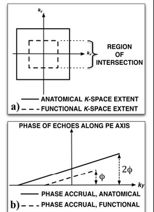
**Figure 2:** Extent in  $k$ -space (a), and ideal phase accrual along  $k_y$  axis (b). Here, the anatomical image has twice the resolution of the functional. For exact co-registration, twice the phase accrual has to occur over the extent of  $k_y$  covered in the anatomical scan.
