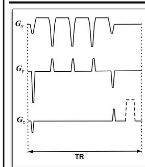
**Figure 1:** 3D Flyback EPI with echo train length 4. The crusher, denoted by the dotted trapezoid, is played out during the anatomical sequence, but not during SSFP fMRI.
