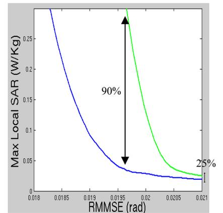
Fig.1: Performance of the pulse Design: global power constraints (green) and local SAR constraints (blue)
