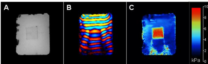
Fig.2 MRI image of the gel phantom with inclusion (A), wave image obtained at 150Hz (B) and the estimated shear stiffness (C).
