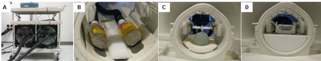
Fig.1 The modified subwoofers are used to deliver acoustic pressure waves into the actuator drivers (A), head actuator (B), probe type actuator (C) and bed type actuator (D).
