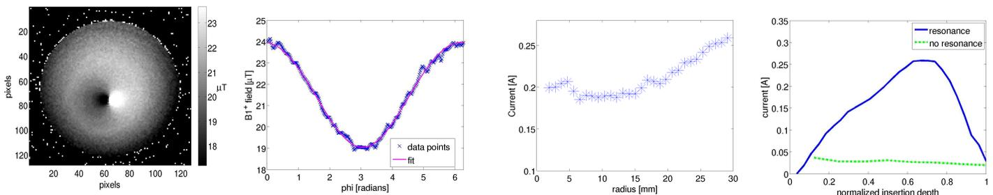
Fig: (1) inhomogeneous  $B_1^+$  map caused by the presence of a conductive wire, (2) measured  $B_1^+$  profile together with a fit, (3) radial dependence of the measured current (radius = 9 mm), (4) current profile along wires for resonant and non-resonant conditions.
