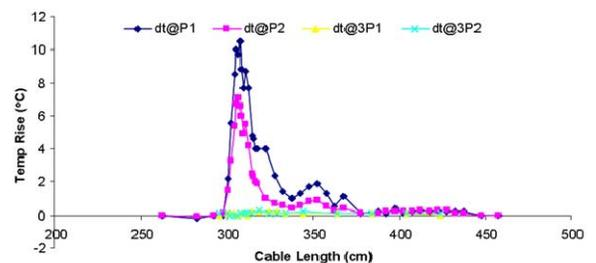
**Figure 3:** A plot of the temperature rise vs. the resonant cable length reveals 1) RF heating is a problem only at some resonant length of the cable and 2) the coaxial cable trap balun effectively eliminates RF heating even in the worst case of a static phantom. In this plot, P1, 3P1 and P2, 3P2 correspond to the tip and matching network regions of the multimode coil with and without baluns respectively.
