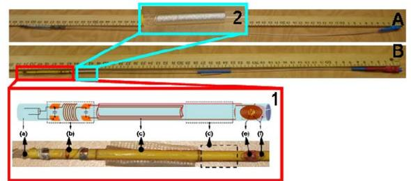
**Figure 1:** Multimode coil implementation without (A) and with (B) coaxial cable trap baluns. The multimode device is magnified and shown in box 1 along with a schematic of the multi-mode coil showing (a) the flexible plastic tube, (b) the  $\pi$  matching network, (c) the 2-turn imaging loop, (d) the region of signal cancellation, (e) the tuning capacitor (yellow rectangle) and (f) the tip tracking Helmholtz pair. A magnified picture of the coaxial cable trap is shown in box 2.
