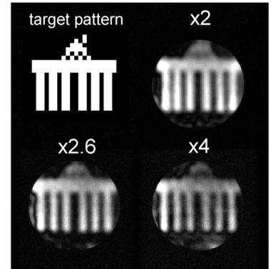
Fig.3: 2D spatially selective PEX experiments in the gel phantom using the <sup>2</sup>CONTAR array and varying acceleration factors.
