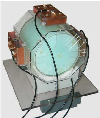
Fig.1: 4-channel <sup>2</sup>CONTAR array and gel phantom (i.d. 20 cm)
