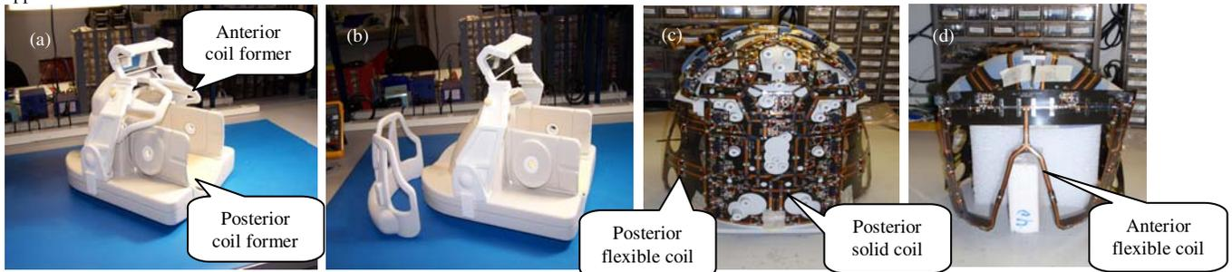
Fig. 1 Mechanic structure and coil configuration of 32ch coil array. (a) Mechanic structure with anterior coil former; (b) Mechanic structure without anterior coil former; (c) Element configuration of posterior coils; (d) Element configuration of anterior coils.
