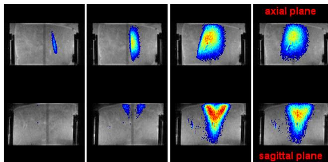
Figure 2. Temperature maps during the slice sonication sequence, at different time frames. From left to right, are being performed the first line, the fourth line, the last line. Finally the post-sonication cooling regime is shown. Minimal focus is 32mm and maximal focus is 69mm.
