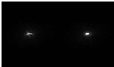
Fig.1. K-space data acquired with SE-DWI sequence (left) and corrected data by shifting odd phase encoding lines by a factor calculated with correlation coefficient (right).
