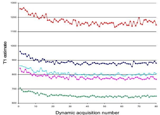
Figure 1. Short-term GRE signal drift for a selection of T1 samples. Each colour represents a different T1 sample (1210, 940, 786, 780, and 625 ms)
