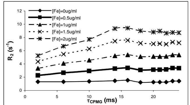
Figure 2.  $R_2$  sensitivity to varied  $\tau_{CPMG}$  for CPMG acquisitions using MPIO/gelatin samples with a range of iron concentrations. Diffusion sensitivity is consistent with Luz-Meiboom predictions.
