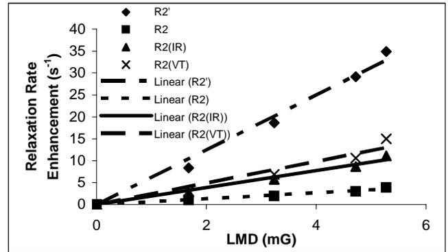
Figure 1. Relaxation rate enhancement of SPIO/gelatin samples as quantified by GE ( $R_2^*$ ), SE ( $R_2$ ), IR bSSFP ( $R_2^{(IR)}$ ) and VT bSSFP ( $R_2^{(VT)}$ ). bSSFP relaxation rates are significantly greater than  $R_2$ , and well correlated to LMD, a measure of SPIO concentration.
