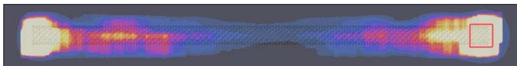
FIG. 2: Exemplary 1.5 T 1g avg. SAR distribution (linear scaling), design-simplified 200 mm stent
