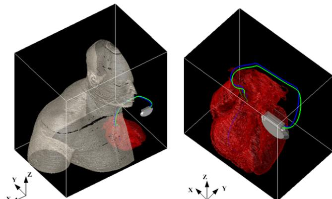
**Fig. 1.** – Sketch of implanted pacemaker in the torso of the tissue equivalent body model; The size of the pacemaker is ~53x43x13 mm.
