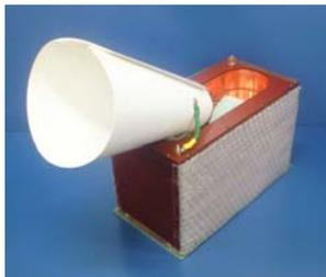
Fig.1 RF probe with local shield
