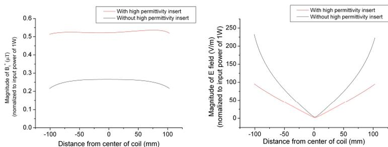
Fig 3. 1D profile of  $B_1^+$  and E field crossing the center of ROI with and without high dielectric insert
