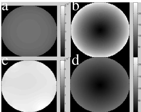
Fig 2.  $B_1^+$  magnitude distribution within ROI without(a) and with(c) high dielectric insert. E magnitude distribution within ROI without (b) and with(d) high dielectric insert
