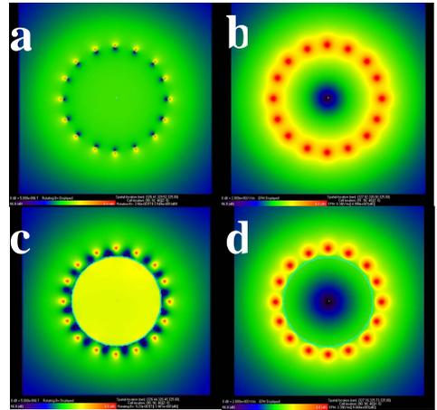
Fig 1.  $B_1^+$  magnitude distribution without(a) and with(c) high dielectric insert. E magnitude distribution without (b) and with(d) high dielectric insert
