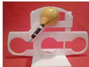
Fig. 3 Gradient field probe secured in bore measurement grid
