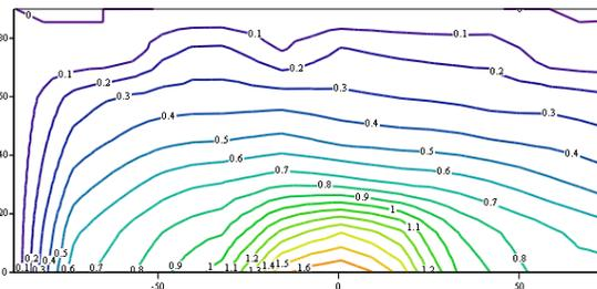
Fig. 5 H-field in the bore, horizontal cut through isocentre, scale in cm with reference to the isocentre
