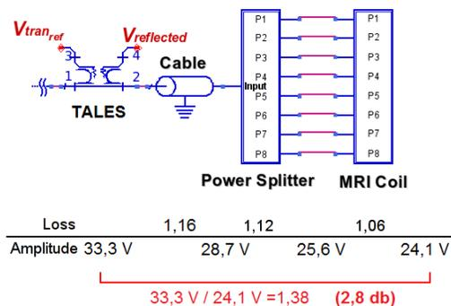
Fig. 1. Circuit between TALES and MRI coil input
