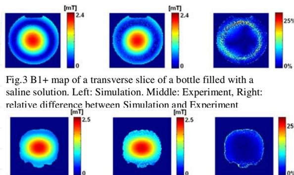
Fig.3 B1+ map of a transverse slice of a bottle filled with a saline solution. Left: Simulation, Middle: Experiment, Right: relative difference between Simulation and Experiment
