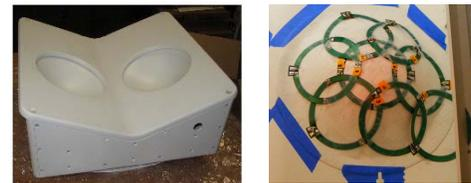
**Figure 2.** a) Finished breast coil housing. b) Coil element layout on custom former.
