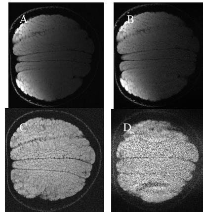
**Figure 3.** Grapefruit phantom [3D 384x256x64] imaged with a) custom coil image and no acceleration [3:56 scan time] b) custom coil with 3.3x acceleration [1:04 scan time] c) industrial coil with no acceleration d) industrial coil with 3.3x acceleration. Acceleration was performed in L/R and S/I directions. Note custom coil has three times SNR in full acquisition images.
