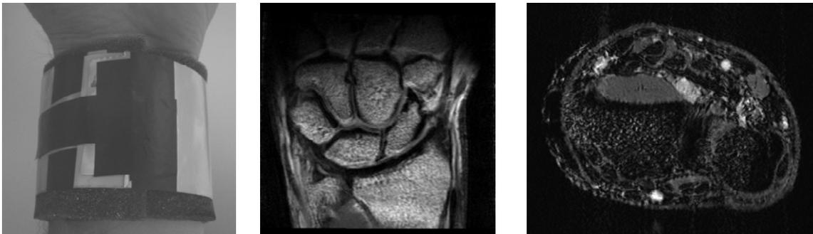
Figure 1. (left) Photograph of the flexible loop-gap resonator wrapped around the left wrist of a volunteer. (centre) Coronal T1-weighted spin-echo sequence acquired (TR/TE 1514/20, 228 x 180 data matrix zero filled to 480x480, fifteen 2 mm slices, flow compensated, 1 signal average). (right) One slice from a high-resolution 3D gradient echo data set (TR/TE 56/5.6 ms, data matrix 400x324x52, spatial resolution 0.18 x 0.18 x 0.4 mm, 1 signal average, 8 minutes data acquisition time).
