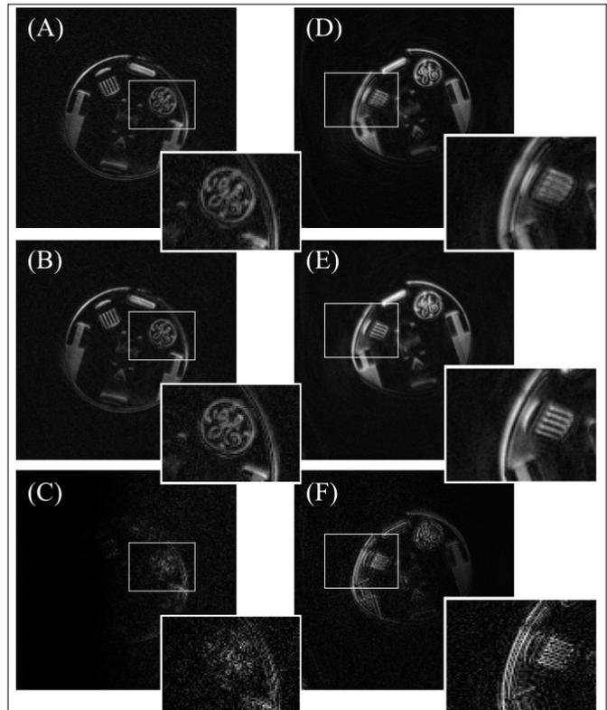
The resolution phantom was scanned in the sagittal orientation. (A), (B), and (C) are with a  $z$  offset of -58 mm acquired with a 4-channel coil. (D), (E), and (F) are with a  $z$  offset of -109 mm acquired with an 8-channel coil. (A) and (D) are the uncorrected images. (B) and (E) are the corrected images using an image domain approach. (C) and (F) are the difference images.
