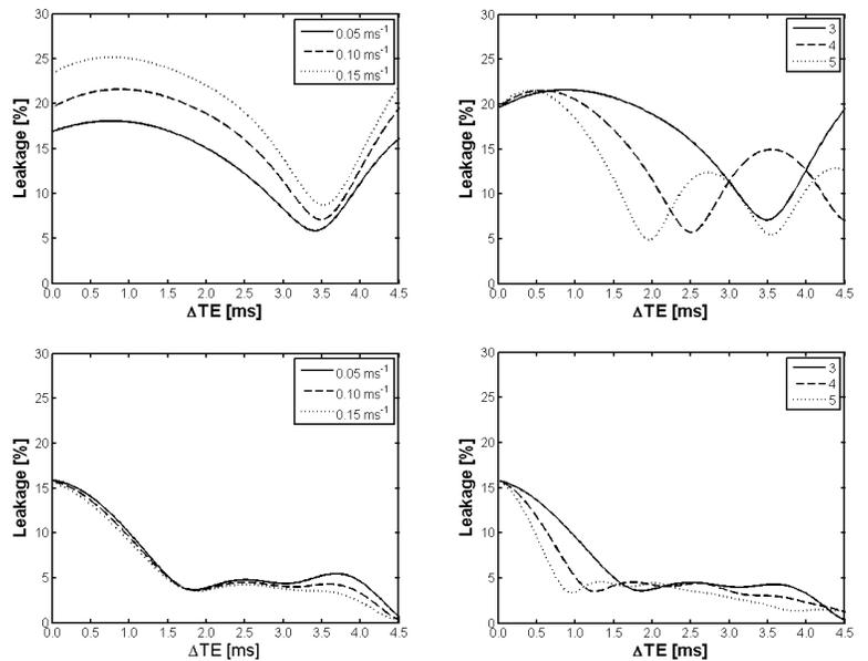
Fig. 2. Relative amount of leakage of fat into water signal as function of the echo spacing  $\Delta TE$  using three echoes and different relaxation rates (left) and three to five echoes and a relaxation rate of  $0.1 \text{ ms}^{-1}$  (right), excluding (top) and including (bottom) relaxation in the signal model for the separation.
