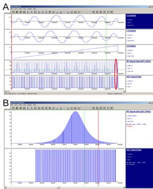
Fig. 1: A) Chronogram of the SWIFT sequence simulated with POET, for 64 directions. B) Zoom on a gapped pulse and related acquisition events included in the red ellipse of 2A.
