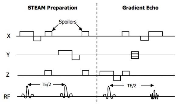
**Figure 1** – STEAM preparation prior to a standard gradient echo sequence for reduced-FOV imaging.
