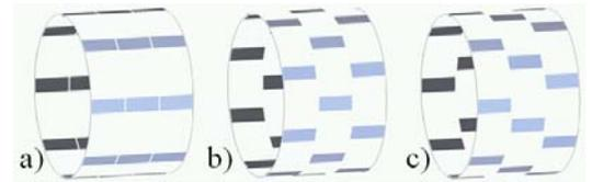
**Fig. 1:** Arrangement of the antennas for a coil with 3 segments and 8 elements per segment. a) all antennas are in line, b) adjacent segments are maximally rotated (angular difference  $22.5^\circ$ ), and c) equal angular distribution of all elements (angular difference  $15^\circ$ ).
