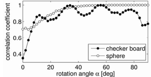
**Fig. 2:** Correlation vs. rotation angle  $\alpha$  for different target patterns. Note that a correlation below 0.8 corresponds to a significant degradation of excitation quality. The oscillations in case of the checker board are due to the high symmetry of the pattern, which leads to preferred directions in  $k$ -space.
