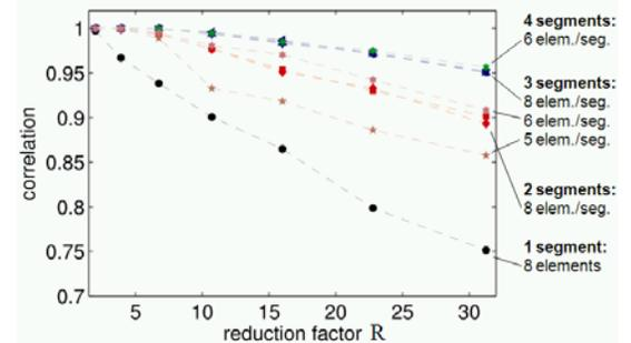
**Fig. 3:** Correlation vs. reduction factor for different coil configurations. More elements result in higher performance. The relative rotation of the segments has no influence on the results.
