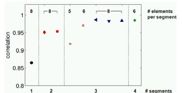
**Fig. 4:** Excitation quality for different coil configurations for a reduction factor of 16. Configurations with equal number of segments and equal number of elements per segment differ by the angular difference between the segments (see Fig. 1).
