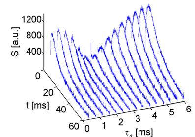
**Fig. 2:**  $^{23}\text{Na}$ -TQF spectroscopy signals of the human head as a function of  $\tau_1$ . Other parameters are:  $\alpha_1 / \alpha_2 = 30^\circ/120^\circ$ ,  $\tau_2 = 0.05$  ms.
