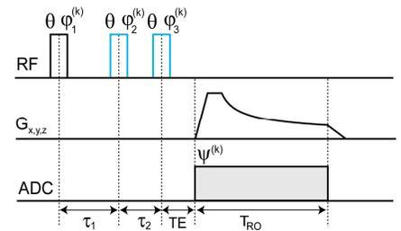
**Fig. 1:** Sequence employed for  $^{23}\text{Na}$ -TQF experiments: three RF pulses with flip angle  $\theta$  and phases  $\varphi_n^{(k)}$ . Delay times between pulses: preparation time  $\tau_1$  and evolution time  $\tau_2$ . Gradient shapes of density-adapted 3D radial acquisition scheme. Acquisition starts after "echo" time  $TE$  with receiver (ADC) phase set to  $\psi_k$  and readout time  $T_{RO}$ .
