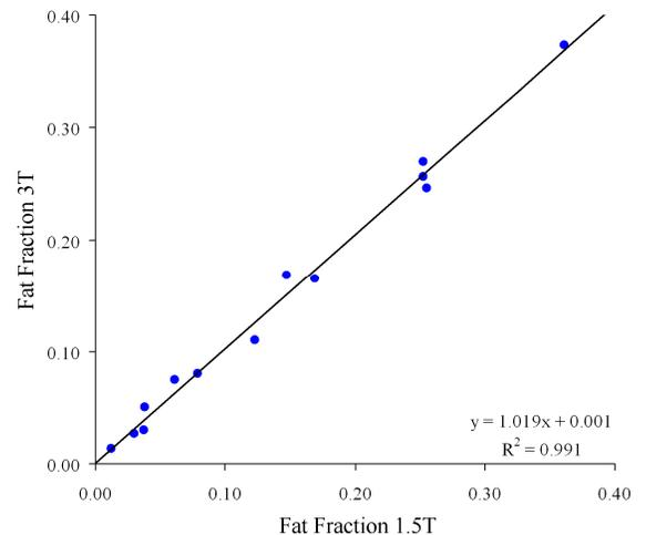
**Figure:** Comparison of the in vivo fat fraction measured at 1.5T to that measured at 3T
