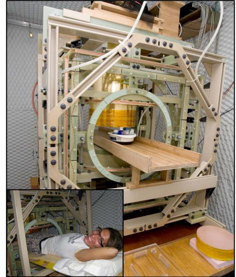
Fig. 1: The custom-built ULF MRI system is capable of imaging any part of the human body for a small adult subject.
