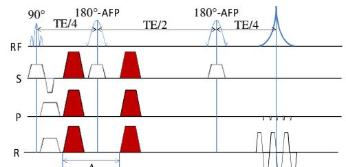
**Figure 1:** Semi adiabatic double spin echo sequence. White: imaging gradients, red: diffusion gradients.
