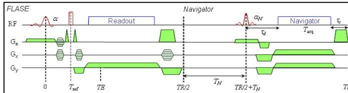
**Fig. 1** 3D FLASE utilizing a selective RF pulse at  $t=0$  and a non-selective refocusing pulse at time  $t=TE/2$ . A selective RF pulse of flip angle  $\alpha_N$  at time  $t=TR/2+T_N$  is applied in a separate slab parallel to the imaging slab, followed by alternating  $x$ - $y$  gradient echo projection navigators [4].
