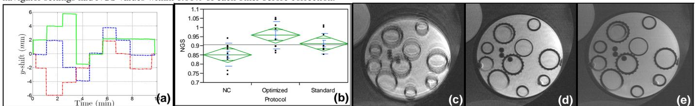
**Fig. 2.** (a) Motion trajectories, (b) Image sharpness for non-corrected images (NC) and motion corrected images for the two navigator settings ( $p=0.003$  and  $0.034$ , respectively). Corrected phantom images: (c) Standard; (d) Optimized, (e) Reference (still), with the NGS values of 0.8753, 1.0548 and 1.0848, respectively.
