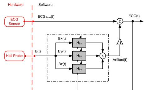
Fig. 2: Flowchart of the artifact reduction method.
