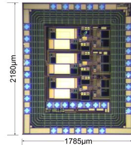
Fig 1: Picture of the 3D Hall Probe chip.
