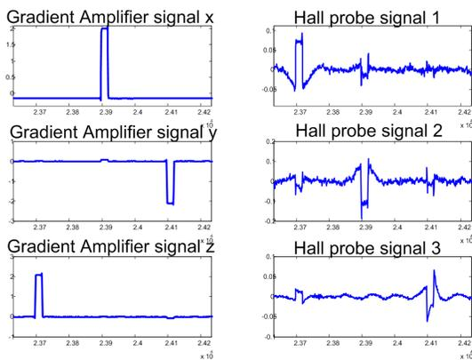
Fig. 3: Comparison of gradient amplifier signals (left) with Hall probe signals (right).
