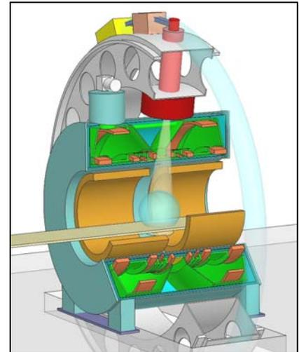
Fig. 1 combined MRI/Linac system
