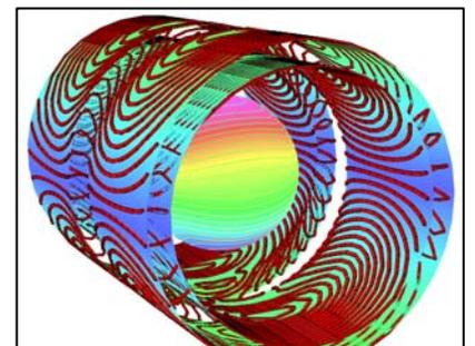
Fig. 3 split gradient coil
