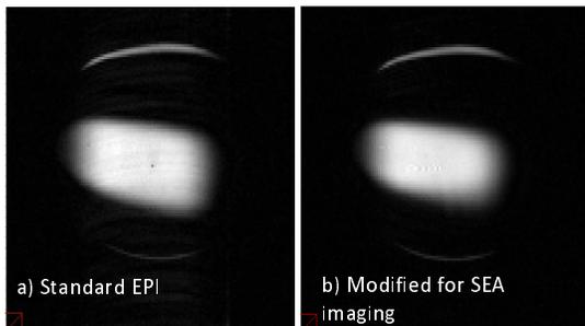
**Figure 3.** (left) Images of a circular phantom with an inner volume selected using a 2D RF pulse from standard blipped EPI approach (Fig 1a) and with a pulse sequence modified to enable SEA imaging during the flyback period (Fig 1b).
