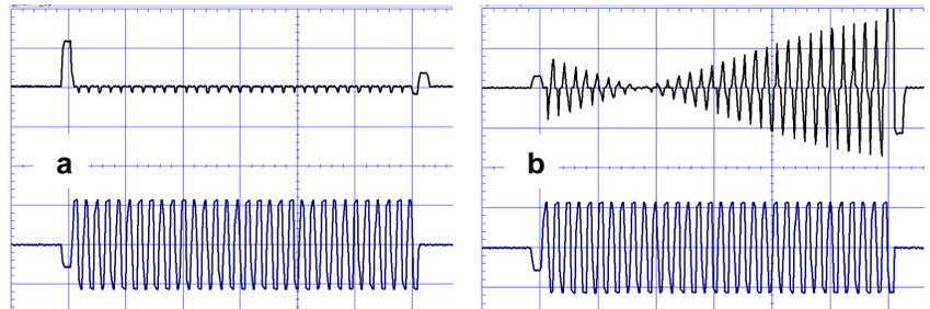
**Figure 1.** Transverse gradients used for a conventional EPI 2D RF pulse excitation (left) and the same sequence modified to enable acquisition of an image during the flyback of the EPI pulse sequence, in between RF pulses. The blipped gradient is not set to the same scale in the two figures. The sequence allows k-space to be traveled along the optimal line needed to compensate for the RF coil phase during each flyback, and then return to the proper position for the RF pulse generation.
