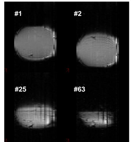
**CONCLUSION:** Combining EPI sequences with RF encoded imaging has the potential to provide MR imaging over the surface of an array sensor at extremely high frame rates, exceeding 1000 frames/second as demonstrated here. This could prove useful in applications such as monitoring fast flow, monitoring ablation or temperature changes in thermal surgery, destructive events, and even RF pulse optimization.
