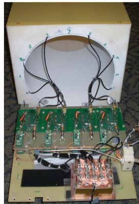
Figure 2. Customized TR eight-coil array configured for four transmitters optimized for imaging the frontal brain. (a)-(c) are the sensitivity maps of the single coils and (d) is for the five coils.
