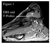
A 400.2 MHz (9.4 T) continuous wave (CW) RF energy (mean SAR = 2.93 W/kg, SD = 0.13 W/kg) was deposited to porcine heads for 1.5 hours using a tuned and matched, four loop, transmit and receive volume head coil. The net average coil input power (forward minus reverse) was measured at the coil by a power meter (Gigatronics Universal Power Meter, model #8652A). The net, whole head average SAR was calculated by measuring the head weight and the total RF power.
