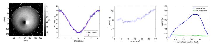
Fig. (1) inhomogeneous B1<sup>+</sup> map caused by the presence of a conductive wire, (2) measured B1<sup>+</sup> profile together with a fit, (3) radial dependence of the measured current (radius = 9 mm), (4) current profile along wires for resonant and non-resonant conditions.
