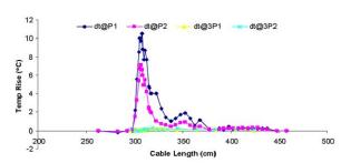
**Figure 3:** A plot of the temperature rise vs. the resonant cable length reveals 1) RF heating is a problem only at some resonant length of the cable and 2) the coaxial cable trap balun effectively eliminates RF heating even in the worst case of a static phantom. In this plot, P1, 3P1 and P2, 3P2 correspond to the tip and matching network regions of the multimode coil with and without baluns respectively.
