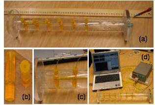
Figure 2: The cylindrical phantom (a) was used to measure the RF heating caused by placing a multimode coil in an external RF magnetic field. The plugs (b) have co-axial and cross axial holes into which, are inserted, respectively the temperature probes and multimode coil (c). The fiberoptic temperature probes are connected to a thermometer that is interfaced with a computer (d).
