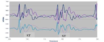
**Figure 3**: Electrode v4 signals prior to (Upper) and post (Lower) processing;  $ECG_{Real}$  (white, from position A),  $ECG_{Real} + V_{MHD}$  (dark purple, from position B),  $ECG_{Real} - V_{MHD}$  (black, from position C). Lower: Averaging signal from positions B and C ( light blue) removes much of the MHD, which is also shown alone (light purple). High-frequency oscillations must still be removed.
