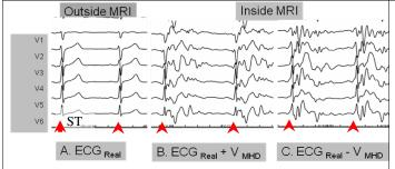
**Figure 2**: 12-lead ECG leads outside the MRI (position A), inside the MRI head first (position B) and inside the MRI feet-first (position C). ECG channels v1-v6 are shown. The QRS complexes are denoted (red arrows) The ST segment in the cardiac cycle is denoted in the left figure.
