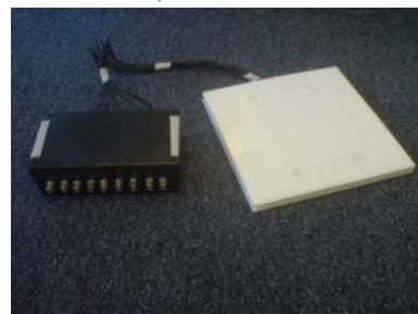
Figure 2. One side of the cube with the RF interface box for testing prior to soldering the Z gradient coil cables and assembling the four sides together.
