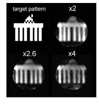
Fig.3: 2D spatially selective PEX experiments in the gel phantom using the <sup>2</sup>CONTAR array and varying acceleration factors.
