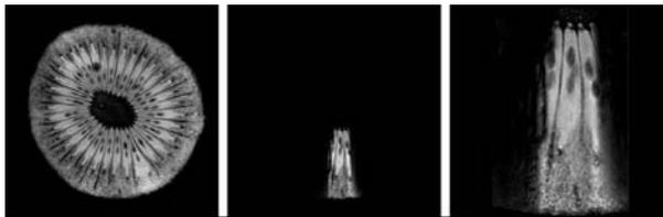
FIG.6. Transmit-sense images of a kiwi.
