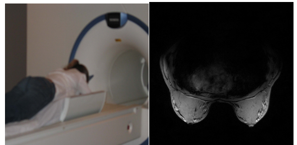
Figure 3: a) Using the bottom six elements of the TEM array as a half-volume transceiver array; b) resulting FLASH image.
