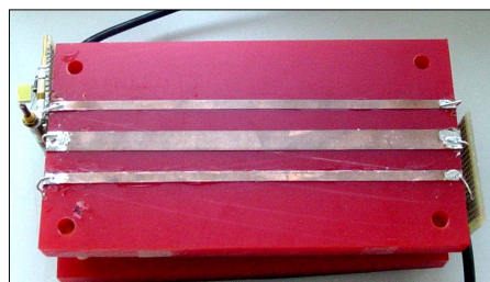
Fig.1: The 4 T double-tuned surface TEM prototype.
