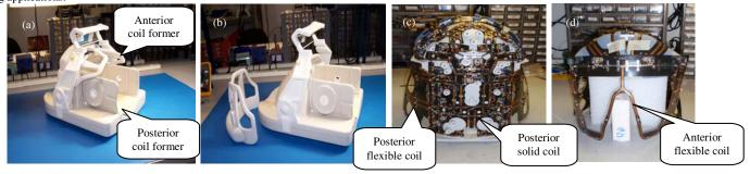
Fig. 1 Mechanic structure and coil configuration of 32ch coil array. (a) Mechanic structure with anterior coil former; (b) Mechanic structure without anterior coil former; (c) Element configuration of posterior coils; (d) Element configuration of anterior coils.
