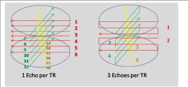
Figure 1: Radial acquisition scheme with 1 echo per TR (left) and 3 echoes per TR(right). The multi-echo sequence can achieve acceleration factor of 2 compared to standard MRA sequence.
