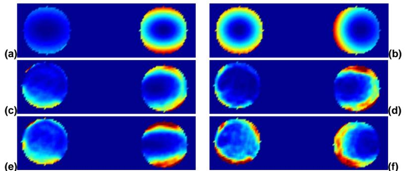
Fig. 1. Local SAR (3). (a) Simulation without and (b) with RF shimming. (c) reconstruction neglecting  $H_{tot}^-$  without and (d) with RF shimming. (e) reconstruction approximating  $H_{tot}^-$  via (6) without and (f) with RF shimming.
