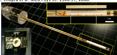
Figure 1: MRI-compatible transurethral heating applicators and motors have been developed for the delivery of this therapy in a closed-bore MR imager (1.5/3.0T).
